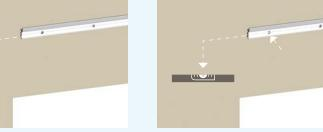
Lign up the profile horizontally and fasten it to the support using all of the
