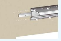
Place the beam on the assembly profile and fasten it to the support using the four holes on the ends.
