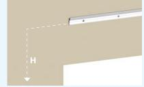
Position the mounting profile at the proper height with respect to the wall.
